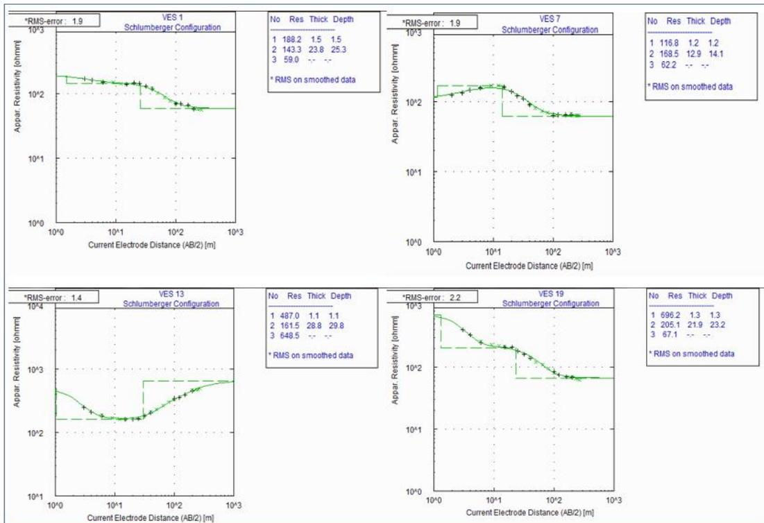
Fig. 3. Resistivity curve for VES 1, 7, 13 and 19 respectively
