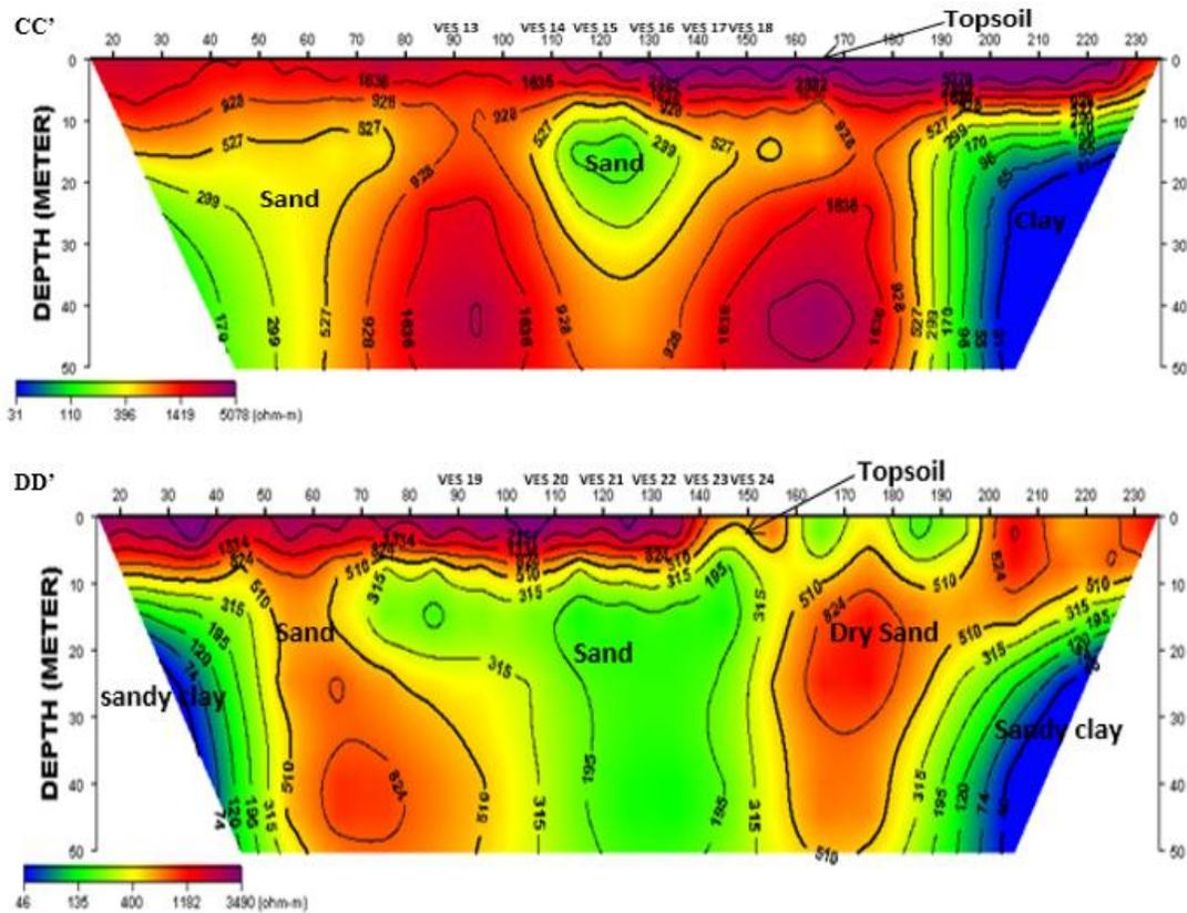
Fig. 6. 2-D Inverted resistivity pseudo-section along traverse  $T_3$  and  $T_4$
