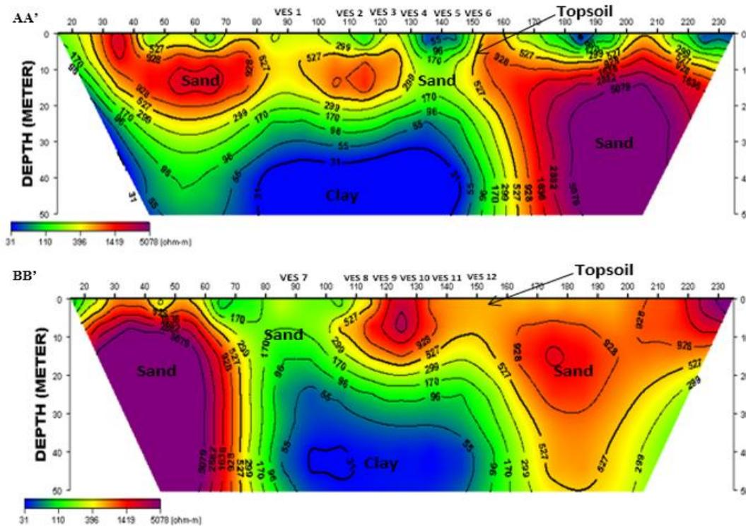
Fig. 5. 2-D Inverted resistivity psuedo-section along traverse T<sub>1</sub> and T<sub>2</sub>
