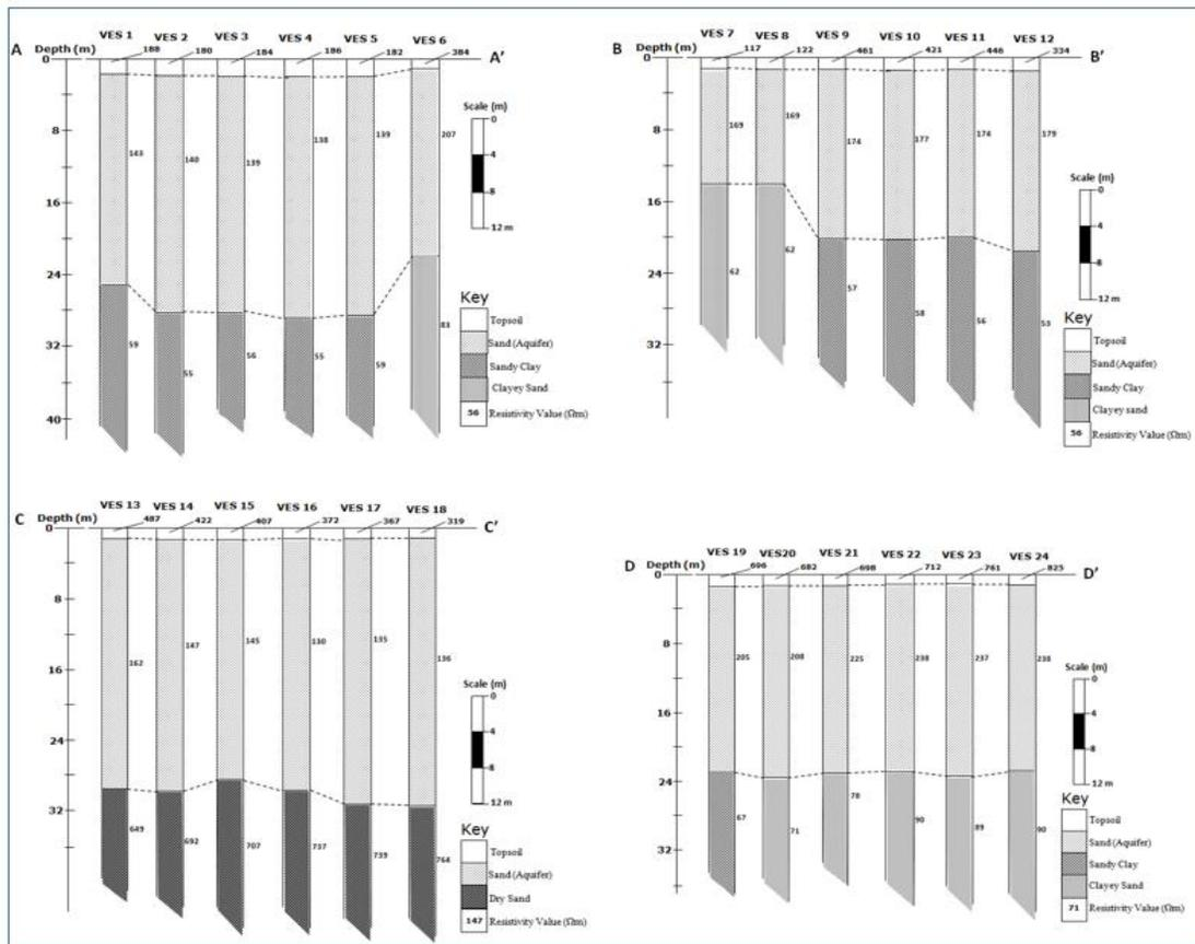
**Fig. 4. Goelectric section of traverse T<sub>1</sub>, T<sub>2</sub>, T<sub>3</sub> and T<sub>4</sub> respectively**
